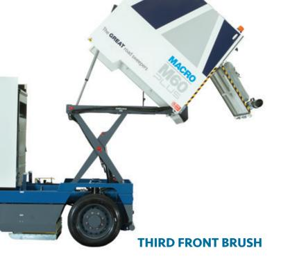
The third front brush can be extended beyond the overall dimensions of the machine, widening the cleaning track and increasing the distance from parked cars, walls, guard-rails, protruding branches etc. to reduce the risk of collisions. In addition, it allows the cleaning of the left side of one-way streets. All these actions are performed easily and intuitively through the joystick on the armrest of the driver seat.
