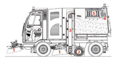
The waste is collected thanks to the mechanical action of the side (1) and central (2) brushes and the vertical conveyor (3). Suction (4) is intended to capture dust as soon as it is raised from the ground. Optimised suction for complete dust suppression thanks to the large surface filter (5).
